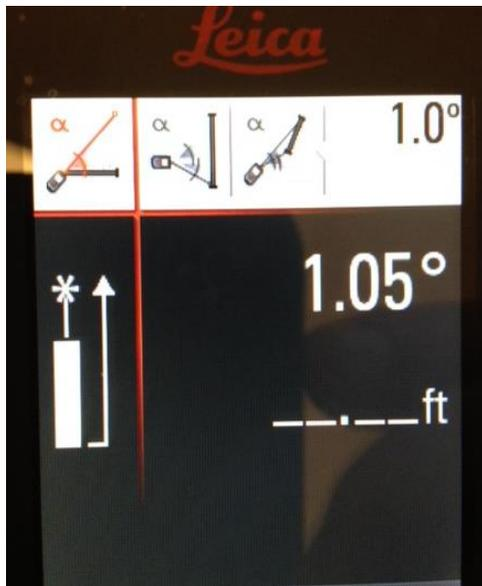
2. Press the Percent button twice in quick succession to the setting "Direct Horizontal Distance". After doing this the graphic will appear as shown in the photo at left with the single red line angling up. You are now ready to take an angled measurement and Disto will calculate the equivalent horizontal measurement. This will
