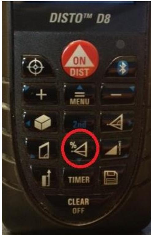
We will explain how to use a Leica Disto D8's "Indirect measurement with tilt sensor". For simplicity, we will call this the "percent button" (shown in the red circle in picture at right). Using the Percent button it is possible to easily measure a horizontal distance inside a bin without actually entering the bin.
