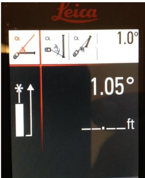
2. Press the Percent button twice in quick succession to measure "Direct Horizontal Distance". After doing this the graphic will appear as shown in the photo at left with the single red line angling up. You are now ready to take an angled measurement and Disto will calculate the equivalent horizontal measurement to the center of the pile (i.e. pile radius) but Disto will ALSO calculate the indirect VERTICAL height which is what we are
