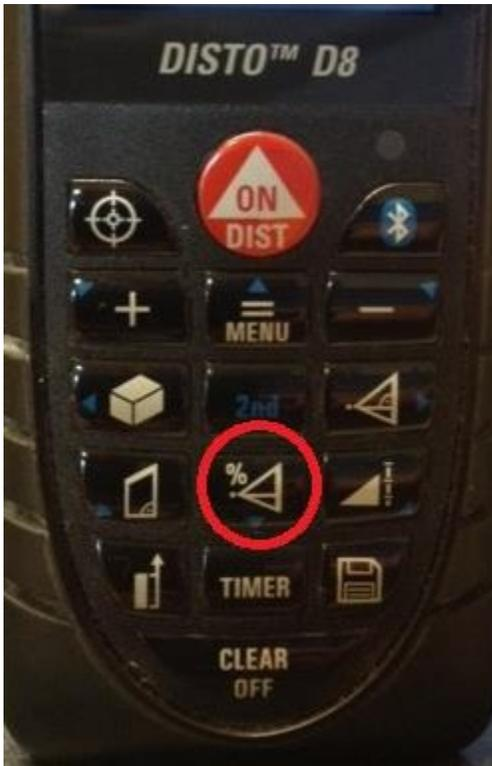
We will explain how to use a Leica Disto D8's "Indirect measurement with tilt sensor". For simplicity, we will call this the "percent button" (shown in the red circle in picture at right). Using the Percent button it is possible to easily measure a vertical height of a ground pile or the sidewall height in a flat building without actually climbing on the grain. 1. Turn the unit on by the pressing the big red button once
